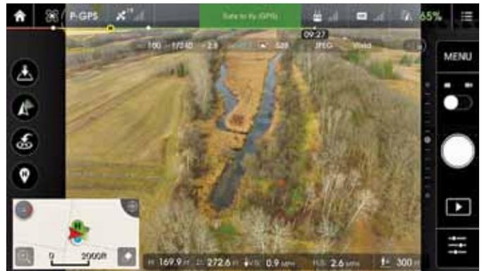
The "DJI Go" application can be downloaded to a smart device and used with a DJI remote control for flying DJI UAS and to monitor and capture live video and imagery.
